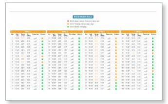
Virtual Service monitoring a rack of batteries using the BPC BACS system. This image shows an alarm on high temperature batteries.
